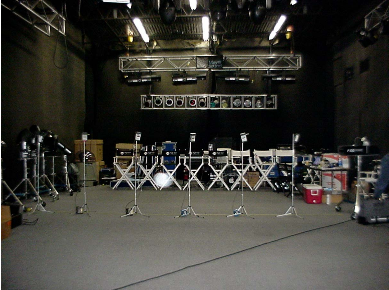
Figure 2. Example sampling configuration consisting of six sampling/monitoring tripods situated at three foot intervals from a smoke machine (far right).
